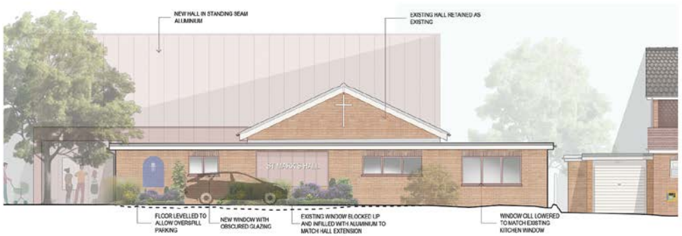
PROPOSED WEST ELEVATION (GREEN TILES LANE) 1:50
